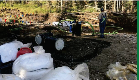
Portable drum vacuum units were used to recover oil in remote locations throughout the release area.
